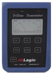
SMPLEX 1T mode displays an analog meter of the voltage between the Black clip and the Red clip (Tip and Ring). The indicated voltage will decrease if a short is applied to the pair at the far-end to confirm the pair identity. Audible beeps are heard if the voltage drop indicates a short.
