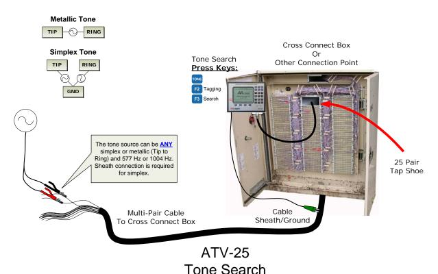
The tone source in the diagram can be any available source capable of 577Hz or 1004Hz tone normally used to tone cable pairs. The ATV-25 will also identify additional pairs that may have cross-coupled tone. In this case, the amplitude of the tone on the pairs is compared and the pair with the highest amplitude is reported as the pair found.
