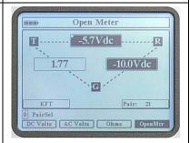
Open meter indicating capacitive distance TG and DC voltages TR and RG.
