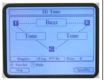
The ATV-25 is sending simplex tone as indicated by the Tone indication on TG and RG. The frequency is 577Hz on PR0. The TR BUZZ confirms a SHORT identification of the correct pair.
