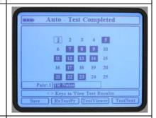
The ATV-25 returns to the test start screen after saving. Start and end pair numbers are incremented for the next 25 pair group. This allows the user to move the tap shoe to the next group and press **[F1] Start** to test the next 25 pair group.
