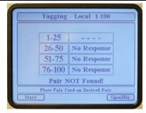
The communications can be confirmed to all the remotes by attempting a pair search without the PRO cord connected. Each Remote
