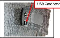
The ATV-25 automatically detects the USB connection and enters the USB Remote mode.
