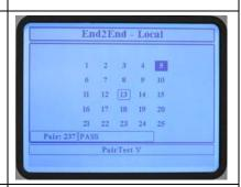
The results are displayed at the end of the test and the first pair of the group is highlighted. The user can use arrow keys ( $\P$ , ightharpoonup, and  $\P$ ) to move the highlight to any pair and view the result. This helps review pairs that have failed. The [F3] **TestViewer** allows the user to see the meter measurements taken during the test.
