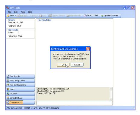
ATV Tools will communicate with the ATV-25 and update the firmware. Progress messages are displayed. The ATV-25 will reset at the end of the process. This is normal.
