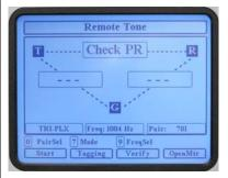
The Verify program was not able to confirm the Tip or Ring. The OpenMtr can be used to determine the status of the pair.
