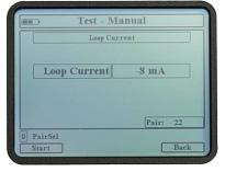
The measured loop current is 8mA. This current is lower than the standard 20mA requirement.
