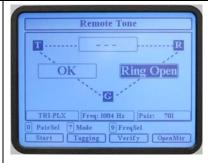
The Tip was found but the ring was not Verified. Tone can be sent on the pair to locate the other side of the pair if the pair is split.
