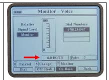
Monitor mode is on, there is no DC voltage on the pair, and no audio as indicated by the 0 – 100 indicator in the middle.
