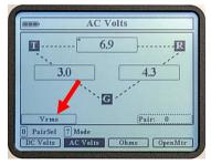
The AC Voltmeter in RMS mode. The readings indicate 6.9Vrms TR, 3.0Vrms TG, and 4.3Vrms RG.
