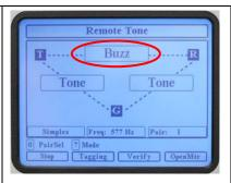
The word BUZZ indicates the ATV R/T has detected a short on the pair.
