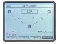
The reading is a typical vacant cable pair the indicated length is 1.79KFT (1,790 feet). The pair is balanced as indicated by the matching TG and RG readings.
