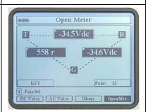
Line voltage is indicated TR and RG. A TG resistance of  $558\Omega$ .
