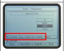
xDSL selection showing Fs = 25.9kHz, Step = 4.3kHz, and Fe = 1.13MHz.
