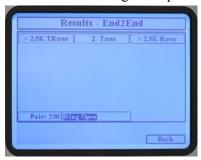
The measurements show a Tip to ground measurement of 2 ohms indicating Tip to Tip continuity. The loop resistance is greater than 2.5K ohms and the Ring to ground resistance is also greater than 2.5K ohms confirming the Ring side is open.
