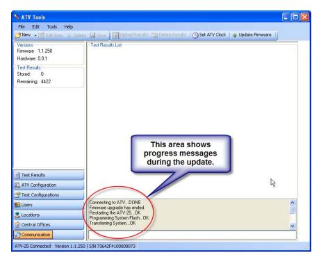
The new firmware version is now displayed in the ATV Tools program. A problem occurred if the version number does not match the new version and the update must be repeated.
