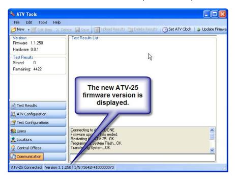
Unplug the USB cord from the ATV-25. The ATV-25 will reset and display the idle screen. The current firmware version is displayed at the top of the screen. This must match the version that was just loaded. Repeat the update if the version number is incorrect.
