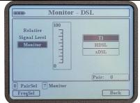
① If the Monitor box is black but you cannot hear any audio, look at the meter, if you see an indication of audio on the line, increase the speaker volume by pressing the [+V] key.
