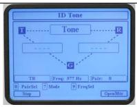
Sending tone TR (metallic), the **9 FreqSel** allows frequency selection
