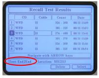
Test results are shown with the last test on top. The highlighted test is an End2End test for the WFD office, Cable 11, Pairs 375 through 400.
