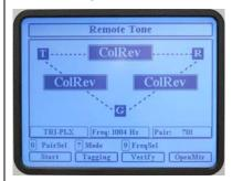
The pair was verified, the Tip and Ring were confirmed but ther is a polarity reversal between the ATV R/T and the ATV-25
