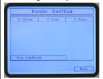
The left arrow, ◀, is pressed in the test viewer to display pair 229. This pair passed. The loop resistance indicates continuity from the Tip at the Local unit through the Remote unit back to the Ring at the local unit.
