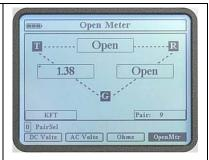
These readings indicate a Ring open condition on pair 9. The Open message indicates that the reading is less than the minimum value of approximately 30 feet.
