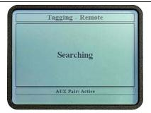
The Remotes receive the tagging commands and searches for the pair. The Remotes return the pair number if the pair is found or "Pair Not Found" if a pair match is not located.
