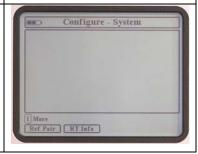
Press the **[F2] RT Info** key. The "Waiting for Remote Unit" and "Connecting" messages will be displayed as the ATV-25 and the ATV R/T connect.
