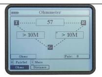
The Ohmmeter **1 More** screen. The reading indicates a 57 ohm short.
