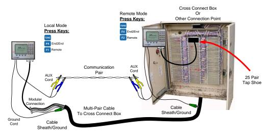
ATV-25 End-to-End Test Configuration
