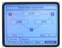
The image shows a vacant, balanced pair that is 3,290 feet long. The Return key is used to return to the Remote Tone mode.
