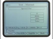
This custom plot configuration shows the Fs set to 990.0kHz and the Step is set to 2.0kHz. The calculated Fe is 1.50Mhz.
