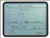
Plot showing an FM signal centered around 1008kHz. Smaller signal spikes are also seen.
