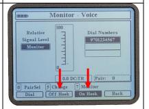
Voice Monitor mode, PR0, Monitor is on, and ATV-25 is on-hook.
