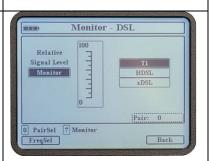
Press **[F1] FreqSel** to enter a specific frequency to monitor. The initial frequency is set to the current mode when the **[F1] FreqSel** key is pressed.
