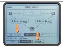
The ohmmeter is converting a 57 ohm short measurement to distance. The indicated distance is 1.1KFT (1,100 feet) at 24ga.
