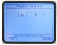
Pair 8 was found by the 1-25 Remote. The PR0 cord is then moved to another pair and **[F1] Start** is pressed to start the tagging process again. Only one Remote was selected in this example.
