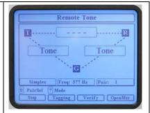
577Hz Simplex tone applied to pair 1. No tone is applied Tip to Ring.
