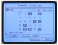
The stored test results are displayed in the same format as the end of testing. This is a review only and the data cannot be changed.
