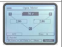
A shorted pair with  $56\Omega$  TR and open indications of 2,860 feet TG and RG.
