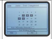
Press **[F2] Save** to save the test results in internal memory. The test results are now available for recall and review on the ATV-25 and for upload to a PC using ATV Tools software.
