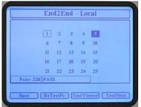
Testing is complete for pairs 226 through 250. Pair 5 is defective.
