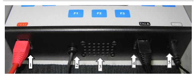
The bottom panel of the D-105 has the connections for the cords and the speaker output grid. The cords are connected according to the labels on the front panel. The cords are identified in the following table.
