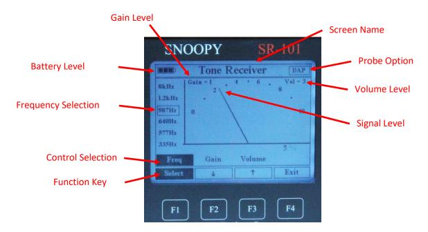
The **F1** key is used to select one of the control options. Function keys **F2** and **F3** decrease or increase the current option. The Gain and Volume values are in the top corners of the analog meter area. The **F4** or **PWR/CLR** keys can be used to exit to the Home screen.
