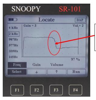
Signal decrease when passing a low resistance fault such as a Short, Ground, or Cross.
