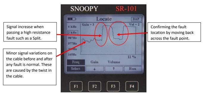
A split location is detected by an increase in signal after the split. Moving the probe back over the fault location verifies the location.
